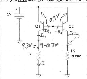
Since  $I_c = I_s(e)$ and since  $I_{s_1} = I_{s_2}$  and  $V_{B_1} = V_{EB_2}$ ,  $I_{c_1} = I_{c_2}$ .
