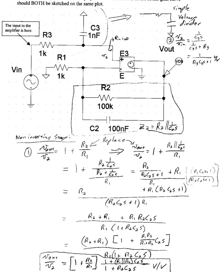
$$\frac{N_{\text{out}}}{V_{\text{in}}} = \frac{0}{V_{\text{o}}} \frac{0}{V_{\text{o}}} = \frac{1}{V_{\text{o}}} \left( \frac{1 + R_1 || R_2 \zeta_2 S}{1 + R_2 \zeta_2 S} \right) \left( 1 + \frac{R_2}{R_1} \right)$$
