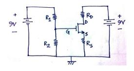
Applying KVL in loop-1,  $V_{th} = V_{GS} + I_D R_S$
