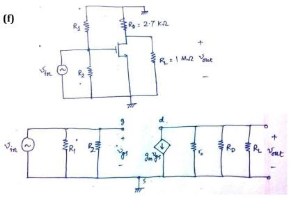
Using the equivalent small signal  $\pi$ -model,
