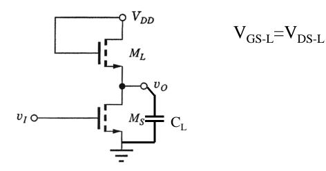
Inverter State: Input is Low Output is High
