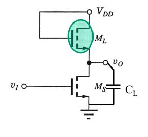
For  $v_i = v_{GS} = V_{OH}$ ,  $M_S$  and  $M_L$  conduct their maximum amount of current.
