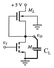
Once again, to insure that  $M_S$  is sufficiently cutoff, we choose  $V_{OL} << V_{TN-S}$  or for our example where  $V_{TN-S}=1$  V,  $V_{OL}=0.25$  V. Thus, when  $v_i=V_{OL}$ ,  $M_S$  is off.
