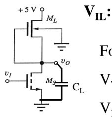
For our numerical example:  $M_{s} = C_{L}$   $V_{TN-L} = -2.23 V$  (>-3V)  $V_{IL} = 1.50 V$
