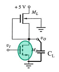
Inverter State: Input is High Output is Low
