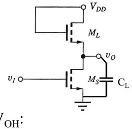
**Inverter State:** Input is Low Output is High
