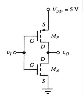
•CMOS Inverter uses one NMOS and 1 PMOS transistor.
