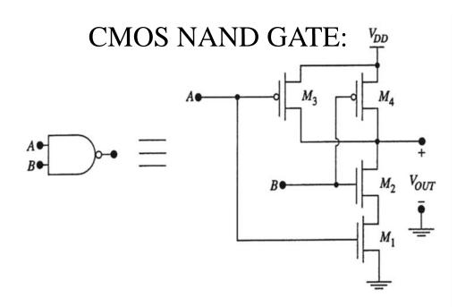
•If both A and B are high,  $M_1$  and  $M_2$  are on, and  $M_3$  and  $M_4$  are off allowing  $V_{out}$  to be pulled low
