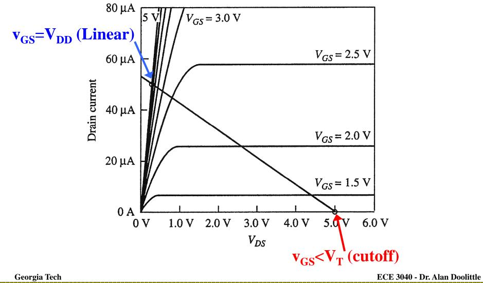
Example: If we wanted the gate to dissipate 0.25 mW using a  $V_{TN}=1V$  and  $K_n'=25e-6 \text{ A/V}^2$ , and having a  $V_{OL}=0.25V$ , what W/L ratio would be needed? What load resistance is required?
