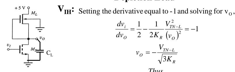
Inverter Transitional State: Input is High Output is Low
