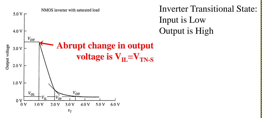
The abrupt nature of this transition is due to  $V_{TN-S} < V_{TN-L}$  due to the body effect. Thus, as  $M_S$  begins to conduct,  $M_L$  is off.
