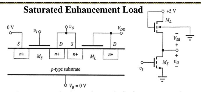
Since the substrate is common to both transistors, the body-to-source voltage,  $v_{SB}$ , varies as the output voltage varies. Thus, the threshold voltage varies resulting in a variation in  $V_{OH}$
