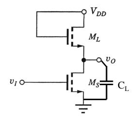
Combining the results from before we see that our Load Transistor is much longer than it is wide, while our switching transistor is wider than it is long.
