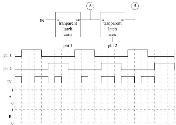
${\bf Part}~{\bf B}$  Complete the following timing diagram for the circuit above. Assume all latch values are initially zero.
