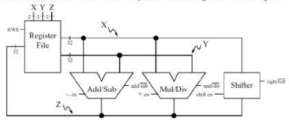
Write microcode for this datapath to compute the function below. The initial values of the registers should be used in the equation. Any register may be modified once its initial value has been used for the last time. Express all signals in octal notation (i.e., to select register two on the X bus, put a "2" in the X column).
