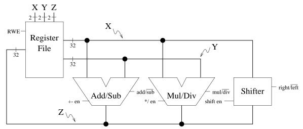
Write microcode for this datapath to compute the function below. The initial values of the registers should be used in the equation. Any register may be modified once its initial value has been used for the last time. Express all signals in octal notation (i.e., to select register two on the X bus, put a "2" in the X column).
