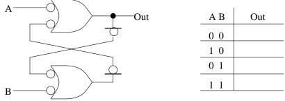
**Part H** Now consider a transparent latch based on this circuit (shown below). How many transistors are used in this implementation (show work)?
