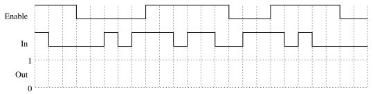
**Part D** Design a latch using four 2-input NOR gates and two inverters. Be sure to label the signals In, Out, and Enable.
