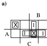
Primes =  $AB, AC, BC, \bar{A}\bar{B}\bar{C}$
