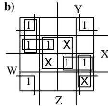
Primes =  $\bar{X}\bar{Z}, XZ, \bar{W}X\bar{Y}, WXY, \bar{W}\bar{Y}\bar{Z}, WY\bar{Z}$
