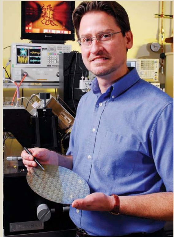
Georgia Tech EE professor John Cressler shows a silicon germanium wafer he is designing to take space circuitry from rad-hard to radiation-immune.
