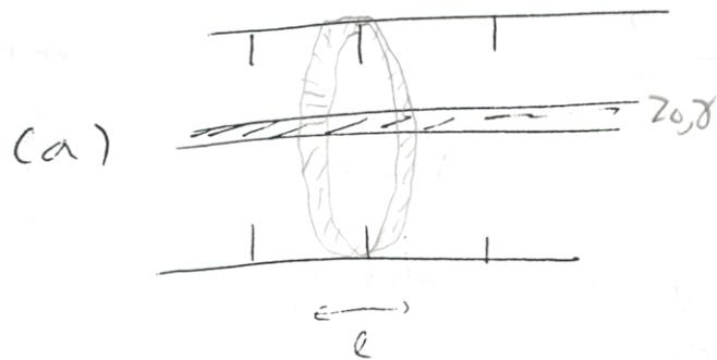
Coaxial line with capacitive disks at intervals  $l$ , inductive loop (small)
