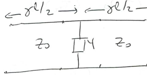
$$\begin{bmatrix} A & B \\ C & D \end{bmatrix} = \begin{bmatrix} \cosh(\frac{\gamma l}{2}) & Z_0 \sinh(\frac{\gamma l}{2}) \\ Y_0 \sinh(\frac{\gamma l}{2}) & \cosh(\frac{\gamma l}{2}) \end{bmatrix} \begin{bmatrix} 1 & 0 \\ 0 & 1 \end{bmatrix} \begin{bmatrix} \cosh(\frac{\gamma l}{2}) & Z_0 \sinh(\frac{\gamma l}{2}) \\ Y_0 \sinh(\frac{\gamma l}{2}) & \cosh(\frac{\gamma l}{2}) \end{bmatrix}$$
