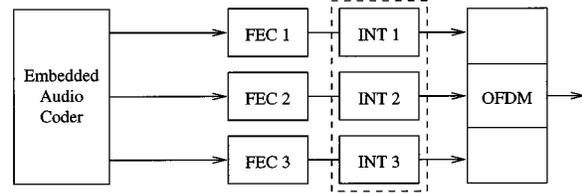
Fig. 24. Conceptual diagram of the multistream transmission system for an embedded audio coder/decoder.
