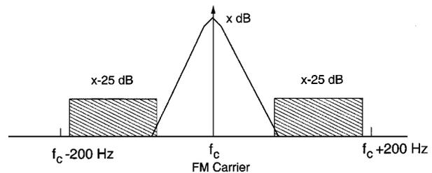
Fig. 18. Basic FM power spectrum.
