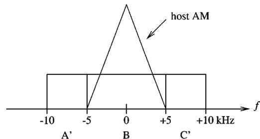
Fig. 26. Conceptual power spectrum for a 20-kHz hybrid IBOC-AM system. The digital data is transmitted in bands A', B, and C' with 1/3 of the total rate in each band.
