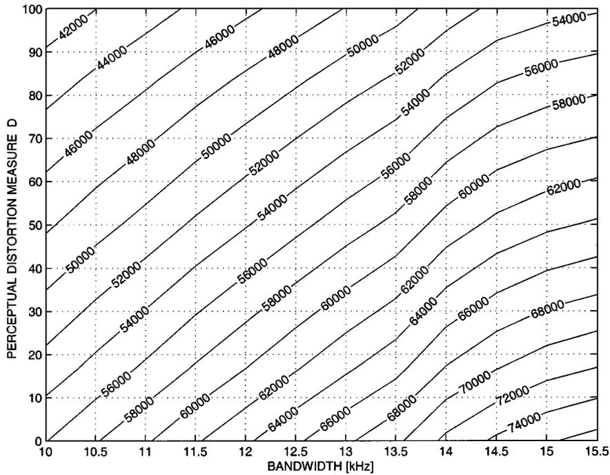
**Fig. 9.** An example of the dependency of the bit rate (indicated on contours in b/s) on the distortion and bandwidth for the PAC audio coder for stereo music signals. Transparent quality corresponds to a value of  $D = 0$ , and “Annoying” quality corresponds to a value  $D = 100$ .
