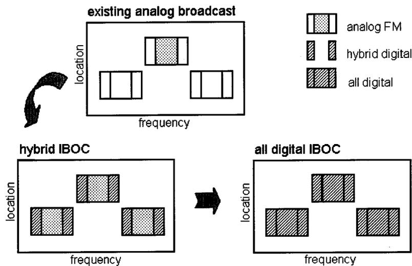
Fig. 17. IBOC transition from analog to digital.
