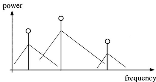
**Fig. 4.** The masked threshold is computed by considering the masking effect of each spectral component of the audio signal.
