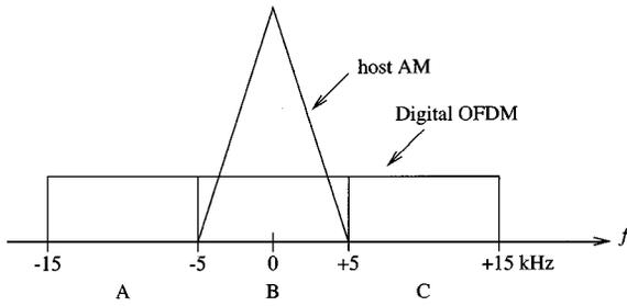
Fig. 23. Conceptual power spectrum of a 30-kHz hybrid 1130C-AM. The digital data is transmitted in bands A-C.
