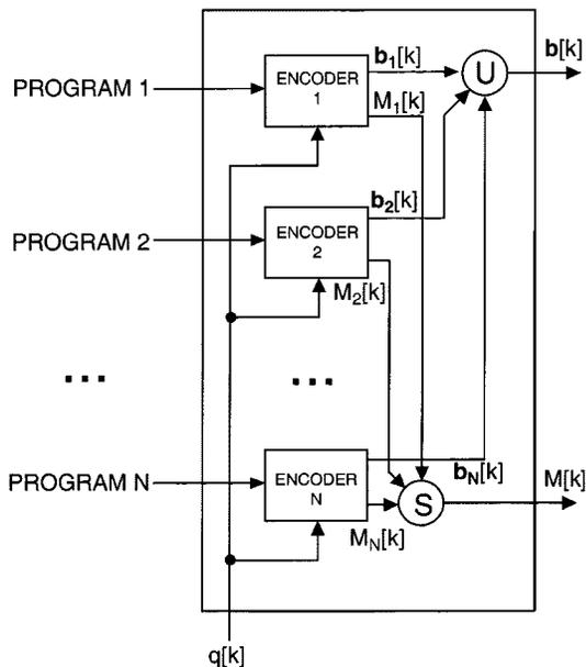
**Fig. 11.** The bitstreams of the  $N$  encoders are combined. The bit rate of a joint frame is  $J[k]$ . A single common distortion criterion is used.
