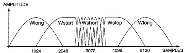
**Fig. 8.** Example for an adaptive window switching sequence in PAC.
