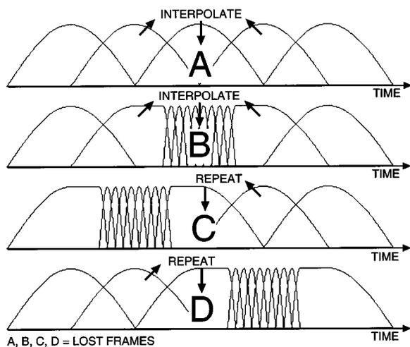
**Fig. 13.** An example of four different cases for mitigating a lost frame.
