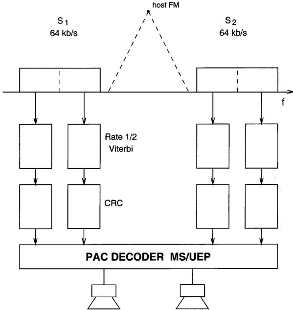
**Fig. 22.** Simplified block diagram for a proposed system based on 64-kb/s multidescriptive PAC and two-level UEP. The multistream transmission is done for four streams and the interleavers are not shown explicitly.
