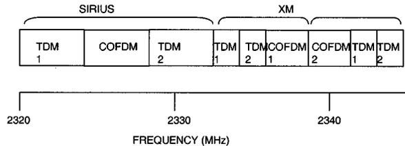
Fig. 31. Allocation of TDM and OFDM bands for XM and Sirius.
