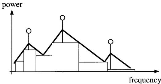
**Fig. 5.** The spectral coefficients are divided into coding bands. Each coding band is quantized such that the error is just below the masked threshold.
