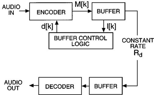
**Fig. 10.** An audio encoder and decoder with a constant bit-rate transmission channel.
