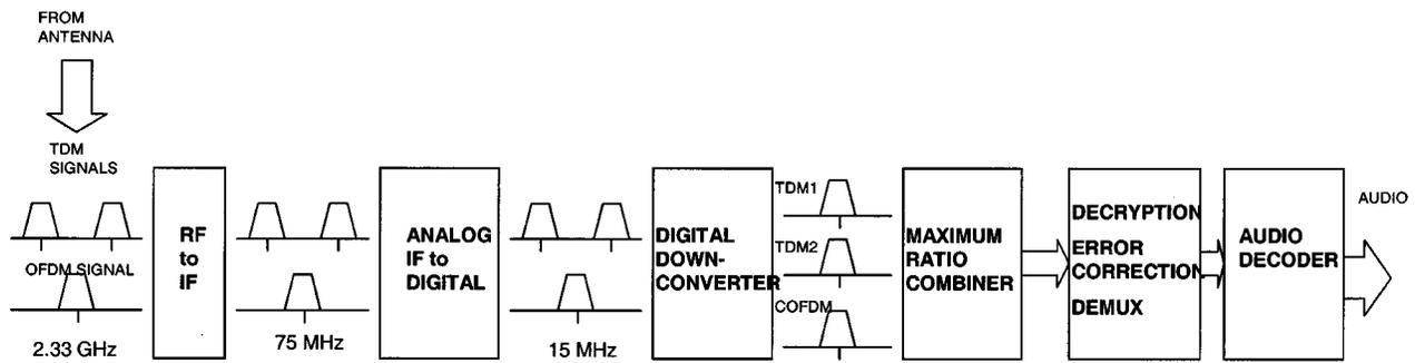
Fig. 30. Decomposition of SDARS receiver chip set.
