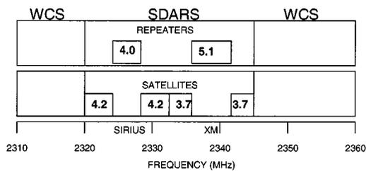
Fig. 29. Frequency-band allocation for SDARS and corresponding bandwidths for repeater and satellite broadcast bands.
