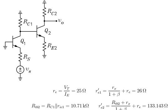
The following solutions are based on the simplified T model. (a) Solve for  $i'_{c1}/v_s$ .
