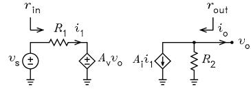
(a) With  $i_o = 0$ , use superposition to write the equations for  $i_1$  and  $v_{o(oc)}$ . Solve the equations for  $v_{o(oc)}$  as a function of  $v_s$ .
