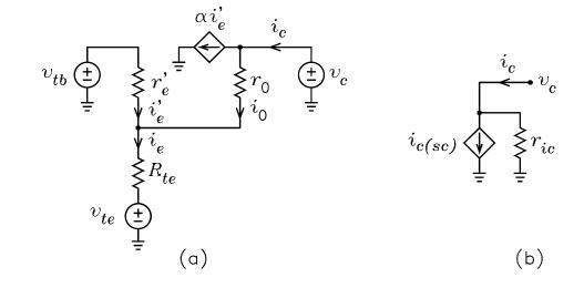
(a) For the circuit of figure (a), use superposition of  $v_c$ ,  $\alpha i'_e$ ,  $v_{tb}$ , and  $v_{te}$  to show that
