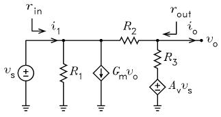
(a) With  $i_o = 0$ , use superposition to solve for  $v_{o(oc)}$  as a function of  $v_s$ .
