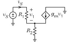
(a) Use superposition of  $v_S$  and  $g_m v_1$  to solve for  $i_S$ .
