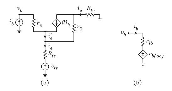
(a) For the circuit of figure (a), use superposition of  $v_{te}$ ,  $i_b$ , and  $\beta i_b$  to show that
