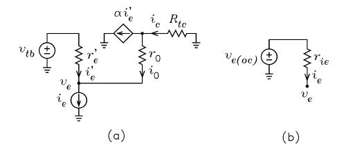
(a) For the circuit of figure (a), use superposition of  $v_{tb}$ ,  $i_e$ , and  $\alpha i'_e$ , to show that
