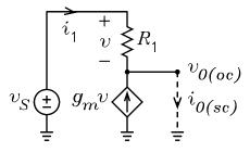
(a) With the output terminals open-circuited, use superposition of  $v_s$  and  $g_m v$  to write equations for  $v_{O(oc)}$  and v. Solve the two equations for  $v_{O(oc)}$  as a function of  $v_s$ .
