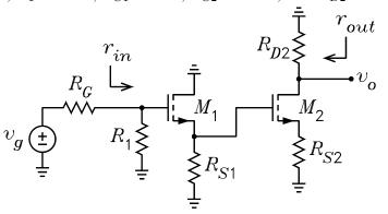
(a) Show that  $g_{m1} = g_{m2} = 1.732 \,\text{mS}$  and  $r_{s1} = r_{s2} = 577.4 \,\Omega$ .
