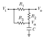
7. Solve for the transfer function for  $V_o/V_i$  for the circuit below. Sketch the Bode plot, label the break frequencies, and label the gain on the zero-slope asymptotes. Answer:
