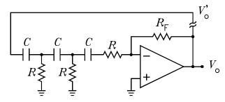
By writing node equations, it can be shown that the loop-gain transfer function is given by
