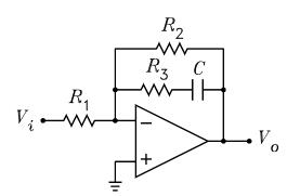
The circuit is to be designed as a lag-lead compensator for a motor control system. The specifications are low-frequency asymptotic gain: -2, input resistance:  $10 \text{ k}\Omega$ , pole frequency: 1 Hz, zero frequency: 10 Hz. Specify the element values. Answers:  $R_1 = 10 \text{ k}\Omega$ ,  $R_2 = 20 \text{ k}\Omega$ ,  $R_3 = 2222.2 \Omega$ , and  $C = 7.1620 \mu \text{F}$ .
