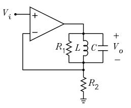
15. For the circuit shown, show that the impedance is real at the frequency
