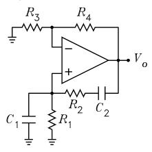
20. The figure shows a phase-shift oscillator with the feedback loop broken.
