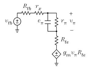
Voltage division can be used to write the equation by inspection for  $v_{\pi}$  as a function of the difference voltage  $(v_{tb} - g_m v_{\pi} R_{te})$ . The pole time constant is the time constant for  $c_{\pi}$ . The equation for  $v_{\pi}$  is
