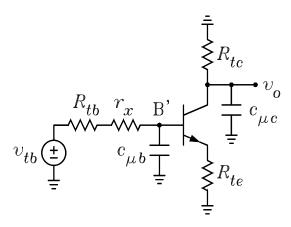
The pole time constant for  $c_{\mu}$  is given by the sum of the time constants for  $c_{\mu b}$  and  $c_{\mu c}$ . Imagine  $c_{\mu b}$  being replaced with an ohmmeter. The time constant for  $c_{\mu b}$  is given by the resistance measured by the
