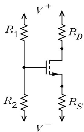
$$V_{GG} := \frac{V_{plus} \cdot R_2 + V_{minus} \cdot R_1}{R_1 + R_2} \quad V_{GG} = -16 \quad V_{SS} := V_{minus} \quad R_{SS} := R_S$$
