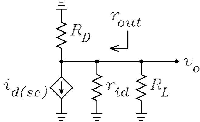
$$K := K_{\text{prime}} \cdot \frac{W}{L} \cdot (1 + \lambda \cdot V_{DS}) \quad K = 2.848 \cdot 10^{-3} \quad g_m := \sqrt{2 \cdot K \cdot I_D} \quad g_m = 3.07 \cdot 10^{-3}$$
