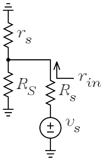
$$r_{in} := R_p(r_s, R_S) \quad r_{in} = 293.85$$
