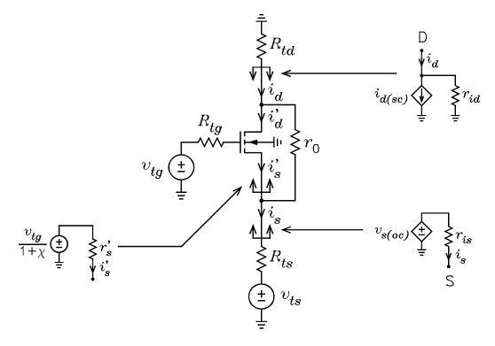
$$i_{D} = K (v_{GS} - v_{TH})^{2} = I_{DSS} \left( 1 - \frac{v_{GS}}{v_{TH}} \right)^{2} \qquad v_{TH} = V_{TO} + \gamma \left( \sqrt{\phi - v_{BS}} - \sqrt{\phi} \right)$$
