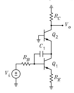
(a) What is the low-frequency gain of the amplifier? Calculate this with  $C_1$  an open circuit.
