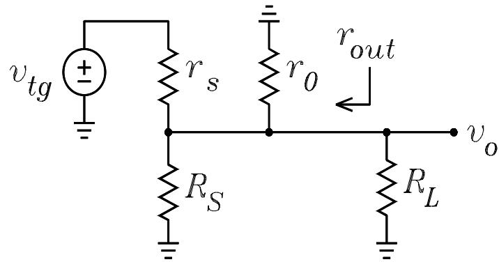
$$v_o := v_{tg} \cdot \frac{R_p(r_0, R_p(R_S, R_L))}{r'_s + R_p(r_0, R_p(R_S, R_L))} \quad v_o = 0.888$$
