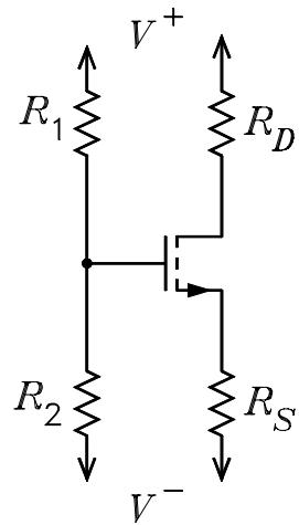
$$V_{GG} := \frac{V_{plus} \cdot R_2 + V_{minus} \cdot R_1}{R_1 + R_2} \quad V_{GG} = -16 \quad V_{SS} := V_{minus} \quad R_{SS} := R_S$$
