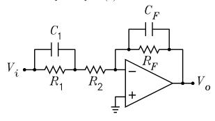
$$\frac{V_o}{V_i} = -\frac{Z_F}{Z_1} = -\frac{\frac{R_F}{1 + R_F C_F s}}{(R_1 + R_2) \frac{1 + R_1 C_1 s}{1 + R_1 \| R_2 C_1 s}} = -\frac{R_F}{R_1 + R_2} \frac{1 + R_1 \| R_2 C_1 s}{(1 + R_1 C_1 s) (1 + R_F C_F s)}$$
