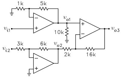
$$v_{o1} = 6v_{i1}$$
