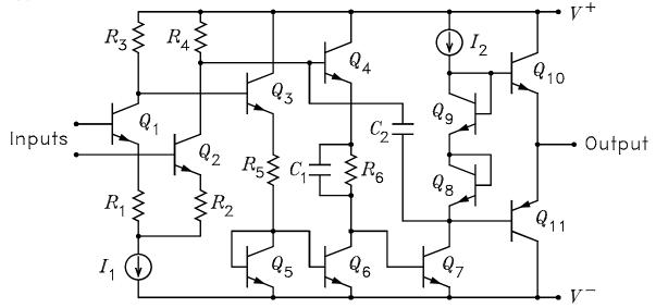
Path 1: Up at  $Q_1$  B, down at  $Q_1$  C, down at  $Q_3$  E, down at  $Q_6$  B, up at  $Q_7$  B, down at  $Q_7$  C, down at  $Q_{10}$  B and  $Q_{11}$  B, down at Output.
