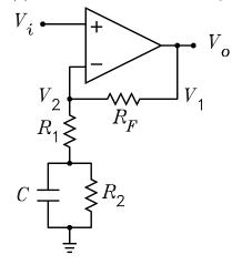
$$A_{low} = 1 + \frac{R_F}{R_1 + R_2} \qquad A_{high} = 1 + \frac{R_F}{R_1}$$
