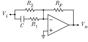
$$\begin{split} A_{low} &= -\frac{R_F}{R_2} \qquad A_{high} = -\frac{R_F}{R_1 \| R_2} \\ \omega_{pole} &= \frac{1}{(R_1 + R_2) \, C} \qquad \omega_{zero} = \frac{1}{R_1 C} \end{split}$$
