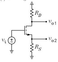
$$v_{o1} = -G_m v_i R_D = -\frac{R_D}{r_s + R_S} v_i = -0.8 v_i$$
