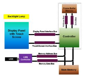
Fig. 3 The proposed architecture of the I-Slate
