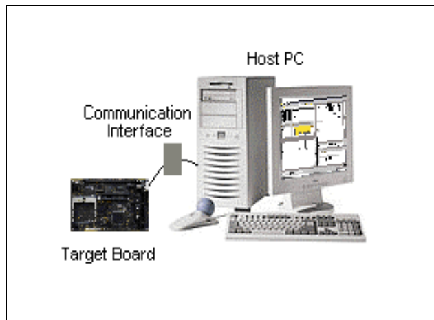
Figure 1. Typical debugging platform for Debugger RTOS applications
