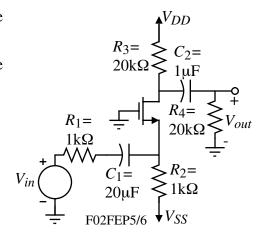
Problem 6 - (20 points - This problem is optional) The FET in the amplifier shown has  $g_m = 1$ mA/V,  $r_d = \infty$ ,  $C_{gd} = 0.5$ pF, and  $C_{gs} = 10$ pF. (a.) Find the midband gain,  $V_{out}/V_{in}$ . (b.) Find the upper -3dB frequency,  $f_H$ , in Hz. (Note: You cannot use the Miller's theorem on this problem because there is no bridging capacitor.)
