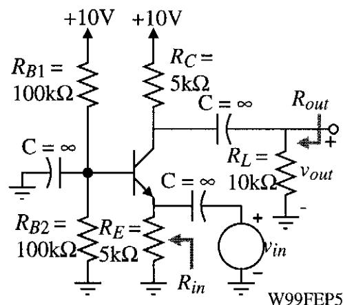
(a.) The circuit used to calculate the collector current is shown. The base current is
