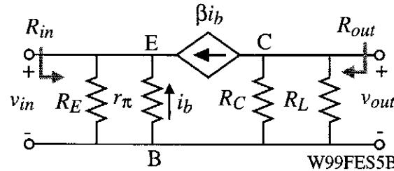
$$i_{in} = \frac{v_{in}}{R_E} - (1+\beta)i_b = \frac{v_{in}}{R_E} + \frac{(1+\beta)v_{in}}{r_\pi} \rightarrow R_{in} = \frac{v_{in}}{i_{in}} = R_E \parallel \frac{1}{g_m} = 24.87\Omega$$
