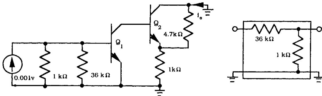
4.) Use the method of feedback analysis to find  $v_2/v_1$ ,  $R_{in} = v_1/i_1$ , and  $R_{out} = v_2/i_2$ .
