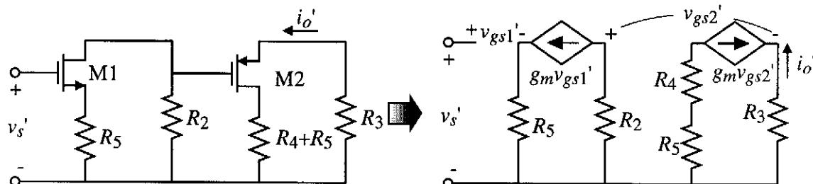
$$A = \frac{i_o'}{v_s'} = \left( \frac{i_o'}{v_{gs2'}} \right) \left( \frac{v_{gs2'}}{v_{gs1'}} \right) \left( \frac{v_{gs1'}}{v_s'} \right) = (-g_m) \left( \frac{-g_m R_2}{1 + g_m R_3} \right) \left( \frac{1}{1 + g_m R_5} \right) = (10^{-3})(-5)(-0.5) = 2.5 \text{ mS}$$
