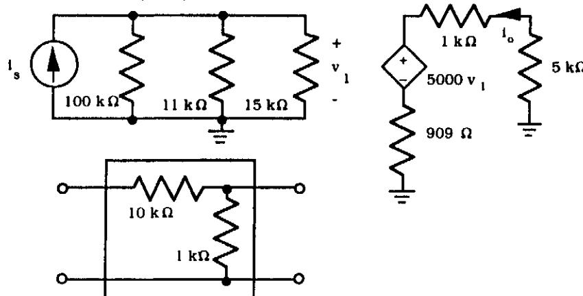
$$R_{IN} = \frac{(100k\Omega \parallel 11k\Omega \parallel 15k\Omega)}{(1 + A\beta)} = \frac{5.97k\Omega}{394} = 15.2 \Omega$$
