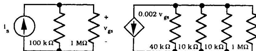
$$y_{11}^F = \left. \frac{i_1}{v_1} \right|_{v_2=0} = 10^{-6} S \quad | \quad y_{22}^F = \left. \frac{i_2}{v_2} \right|_{v_1=0} = 10^{-6} S \quad | \quad y_{12}^F = \left. \frac{i_1}{v_2} \right|_{v_1=0} = -10^{-6} S$$
