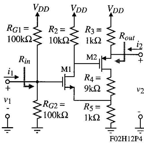
$$z_{11F} = \frac{v_{1F}}{i_{1F}} \mid i_{2F}=0 = R_5 = 1\text{k}\Omega$$
