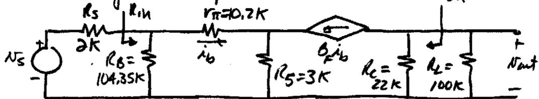
$$R_{in} = R_B \parallel [r_{\pi} + (1 + \beta_F) R_E] = 104.35k \parallel 313.2k = \underline{\underline{78.3k\Omega}}$$
