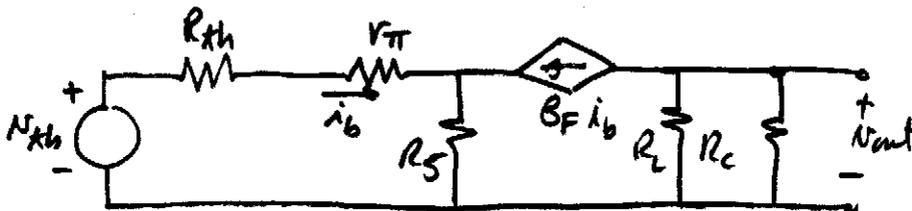
$$R_{Th} = R_s \parallel R_B = 1.96k\Omega \approx R_s$$
