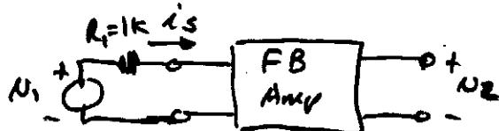
$$\frac{N_2}{N_1} = \left(\frac{N_2}{i_2}\right) \left(\frac{i_2}{N_1}\right) = A \frac{1}{R_{in}} = -\frac{49.9k}{1099\Omega} = -\underline{\underline{45.4V/V}}$$
