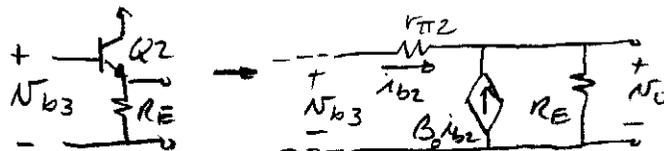
$$N_o = i_{b2} (1+\beta_o) R_E = \frac{N_{b2}}{r_{\pi 2} + (1+\beta_o) R_E} \times (1+\beta_o) R_E \rightarrow \frac{N_o}{N_{b2}} = \frac{(1+\beta_o) R_E}{r_{\pi 2} + (1+\beta_o) R_E}$$
