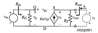
Obviously,  $R_{in} = R_G = R_1 || R_2$ . For  $R_{out}$  we apply the voltage source,  $v_t$ , and set  $v_{in} = 0$  and solve for  $v_t/i_t$  which equivalent to  $R_{out}$ .
