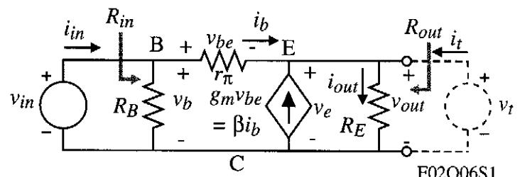
$$R_{in} = R_B \parallel [r_\pi + (1 + g_m r_\pi) R_E] = R_B \parallel [r_\pi + (1 + \beta_F) R_E]$$
