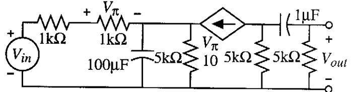
$$\omega_L \approx \sqrt{(507)^2 + (100)^2 - 2(2)^2} = 517 \text{ rads/sec} \Rightarrow f_L = 82.3 \text{ Hz}$$
