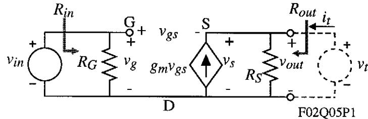
Obviously,  $R_{in} = R_G = R_1 \parallel R_2$ . For  $R_{out}$  we apply the voltage source,  $v_t$ , and set  $v_{in} = 0$  and solve for  $v_t/i_t$  which equivalent to  $R_{out}$ .
