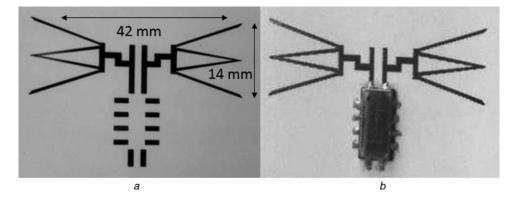
**Fig. 5** *Photograph of the inkjet printed antenna and circuit and photograph of the same printed sample with the mounted SAW based RFID a* Antenna
