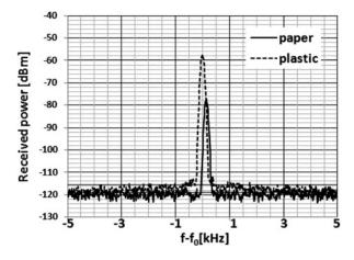
**Fig. 11** Received signal spectrum at  $2f_0 = 7$  GHz: comparison between paper TAG and (prior) PCB design
