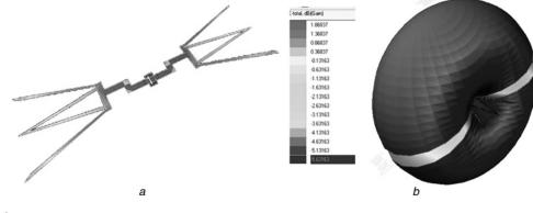
Fig. 7 SAW-based RFID tag a Current density b 3D radiation pattern
