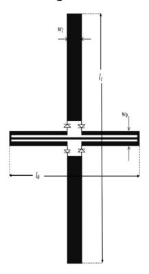
**Fig. 8** Layout of the crossed-dipole frequency-doubling tag operating between  $f_0 = 3.5$  GHz (interrogating frequency) and  $2f_0 = 7$  GHz (tag response)
