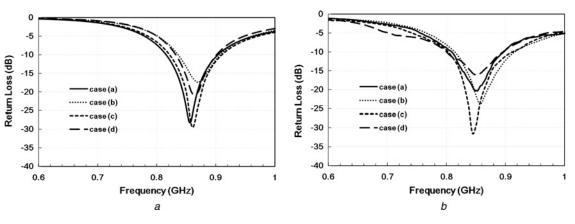
**Fig. 2** *Return loss comparison of the four inkjet-printed antenna designs at European RFID band a* Simulated *b* Measured
