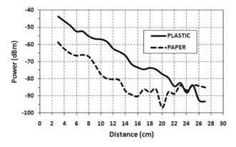
**Fig. 12** Received power against the distance for the crosseddipole frequency-doubling tag
