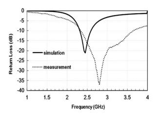
Fig. 6 Return loss of the SAW-based RFID tag Comparison between electromagnetic simulations and measurements
