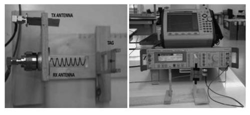
Fig. 10 Measurement set-up for the frequency-doubling tag
