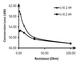
**Fig. 16** Conversion loss trend for different resistance and inductance values ( $P_{in} = -30 \text{ dBm}$ )
