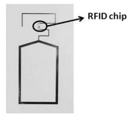
**Fig. 4** *Photograph of the proposed inkjet-printed RFID tag on paper-based substrate with ink-usage after the ink optimisation*
