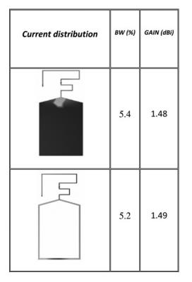
Fig. 3 Topology of inkjet-printed monopole designs of a commercial tag at US RFID band
