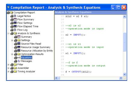
Figure 20. Compilation report showing the synthesized equations.
