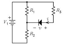
$$V_S = V_1 \frac{R_1}{R_1 + R_2} = 10 \text{ V}$$
