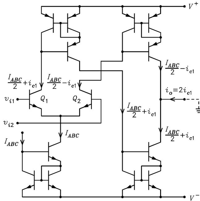
6. The transconductance op amp of problem 5 is to be connected to a current-to-voltage converter as shown below.
