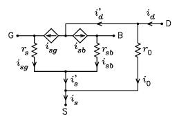
Figure 1: T model of the MOSFET.
