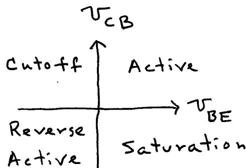
In the active mode, the B-E junction is forward biased. The C-B junction is reverse biased. The labeled current directions are for the active mode. For the PNP device, the current directions are reversed.
