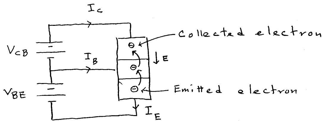
Electrons are emitted from the emitter region across the forward biased B-E junction into the base region. The E field across
