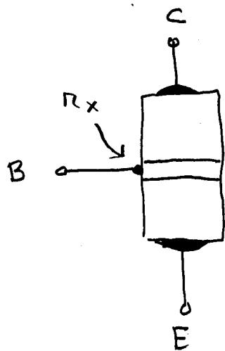
The base region is narrow and its ohmic contact is small. Its resistance is denoted by  $R_x$ .
