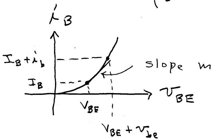
Draw a tangent line at the point  $(V_{BE}, I_B)$ . The slope of the line
