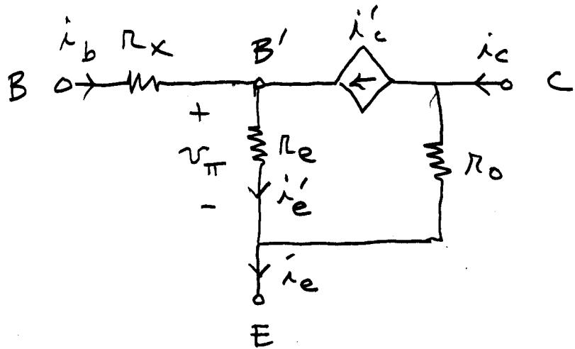
$$i'_c = g_m V_{\pi} = \beta i_b = \alpha i'_e$$
