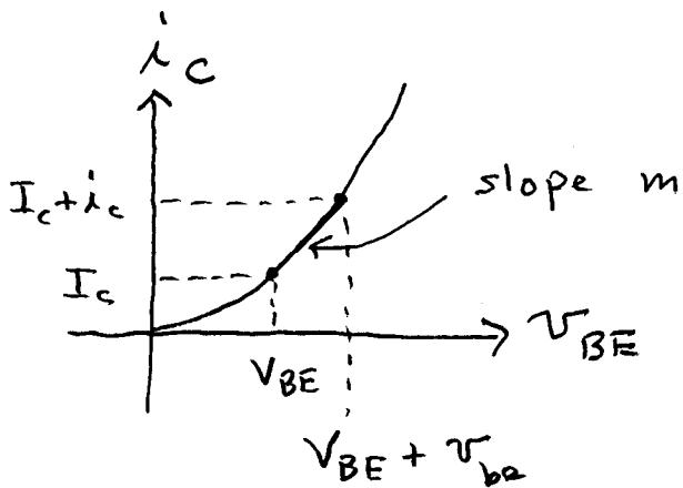
Draw a tangent line at the point  $(v_{BE}, i_C)$ . The slope of the line can be used to relate changes in  $i_C$  to changes in  $v_{BE}$ .
