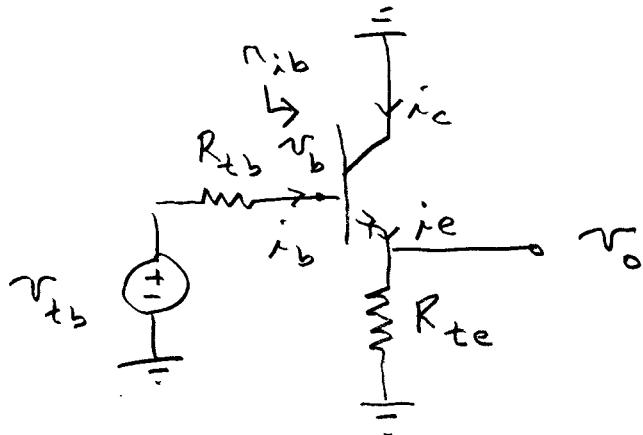
$$v_o = i_e R_{te} = \frac{i_c}{\alpha} R_{te} = g_m (v_b - v_o) \frac{R_{te}}{\alpha}$$
