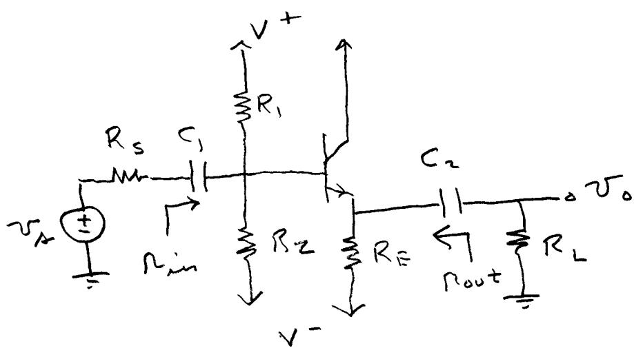
The dc bias currents and voltages are solved for in the same way as for the CE and CB amplifiers. For the ac small-signal solution, set  $V^+ = V^- = 0$  and assume the capacitors are ac short circuits. The circuit reduces to
