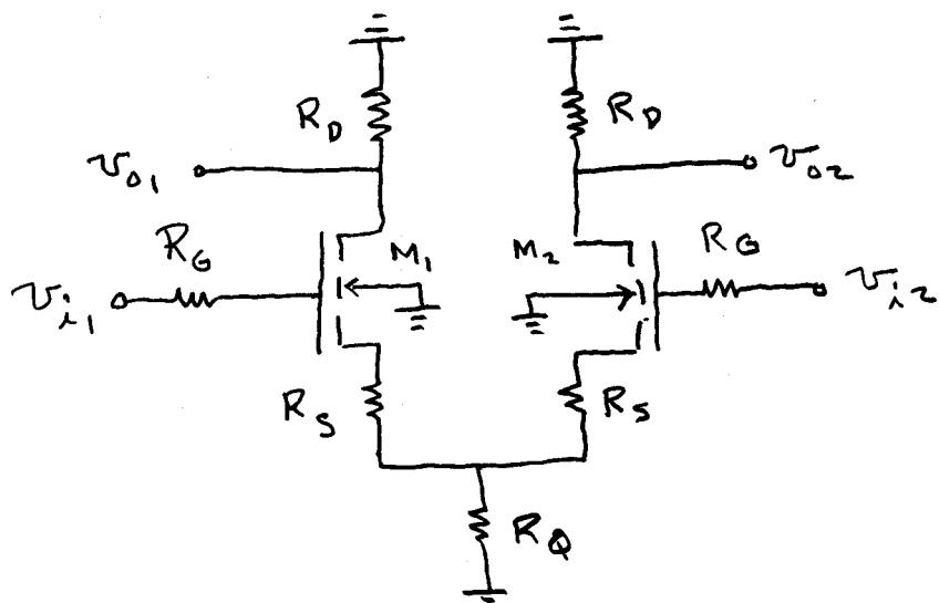
To solve for  $v_{o1}$ , replace  $M_2$  with its Thévenin source circuit. The circuit becomes
