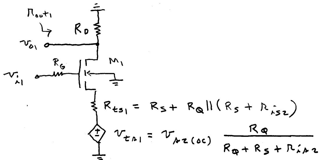
To solve for  $v_{o1}$  and  $R_{out1}$ , replace  $M_1$  with its Norton drain circuit. The circuit becomes
