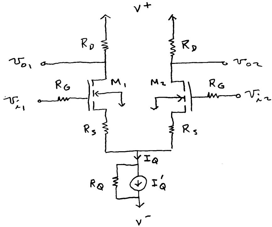
For the dc analysis, set  $V_{i1} = V_{i2} = 0$  and split the source tail supply into two parallel sources -  $I'_Q/2$  in parallel with  $2R_Q$ . For identical devices, the equivalent circuit for either  $M_1$  or  $M_2$  is
