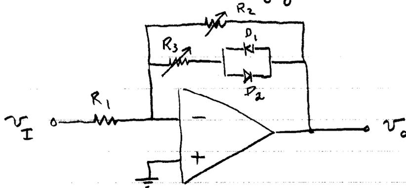
If  $R_3 = \infty$ , the circuit is an inverting amplifier with gain
