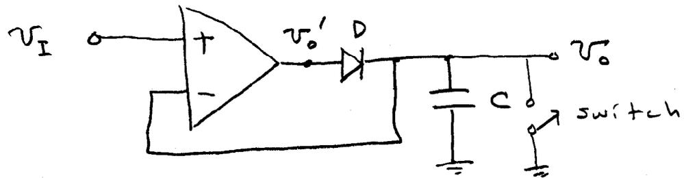
$v_I < v_o \Rightarrow D$  OFF, the op amp loses feedback  $\Rightarrow v_o' = -V_{SAT}$ .
