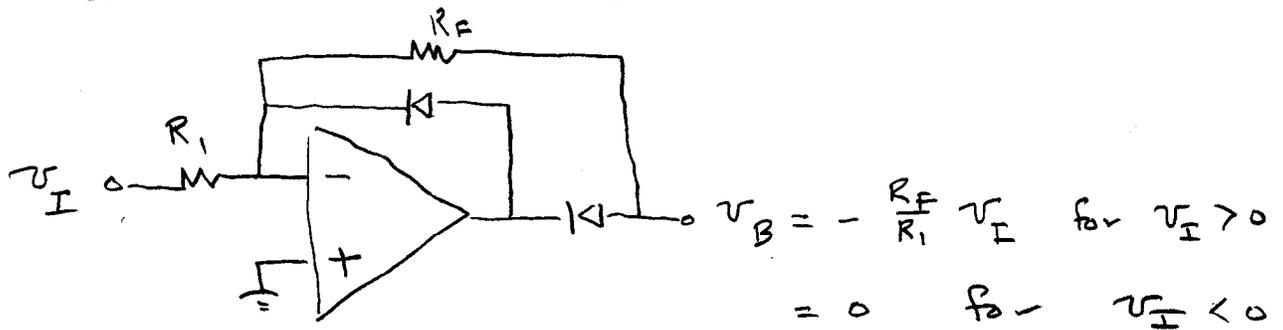
$$\begin{aligned} \text{Let } R_F &= 2R_1 \\ \Rightarrow V_B &= -2V_I \text{ for } V_I > 0 \\ &= 0 \text{ for } V_I < 0 \end{aligned}$$
