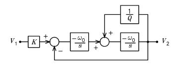
Figure 3: Possible realization for  $G_2(s)$ .
