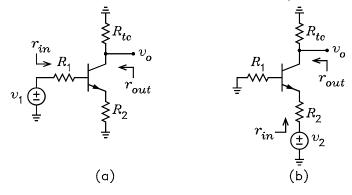
(a) For the CE amplifier of Fig. (a), it is given that  $R_1 = 1 \text{ k}\Omega$ ,  $R_2 = 50 \Omega$ , and  $R_{tc} = 10 \text{ k}\Omega$ . Show that  $I_{C(opt)} = 228 \,\mu\text{A}$ . For  $I_C = I_{C(opt)}$ , show that  $v_o/v_1 = -51.4$ ,  $r_{in} = 16.2 \text{ k}\Omega$ ,  $r_{out} = 8.76 \text{ k}\Omega$ ,  $v_{ni}/\sqrt{\Delta f} = 4.4 \text{ nV}/\sqrt{\text{Hz}}$ , F = 1.21, and NF = 0.829 dB.
