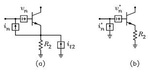
3. The figure shows the ac signal circuits for single stage CE and CB amplifiers. The transistor parameters are  $\beta = 100$ ,  $r_x = 40 \Omega$ ,  $r_0 = 50 \text{ k}\Omega$ , and  $V_T = 25 \text{ mV}$ . (The formulas for the voltage gain, input resistance, and output resistance of the CE and CB amplifiers are given in Section 7.6 of the class notes. You do not have to derive these.)
