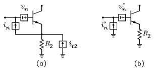
3. The figure shows the ac signal circuits for single stage CE and CB amplifiers. The transistor parameters are  $\beta = 100$ ,  $r_x = 40 \Omega$ ,  $r_0 = 50 \text{ k}\Omega$ , and  $V_T = 25 \text{ mV}$ . (The equations for the voltage gain, input resistance, and output resistance of the CE and CB amplifiers are given in Section 7.6 of the class notes. You do not have to derive these.)
