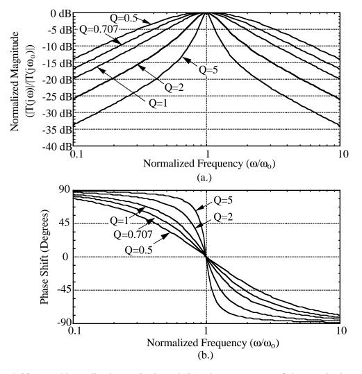
Figure 1-20 - (a.) Normalized magnitude and (b.) phase response of the standard secondorder, bandpass transfer function with Q as a parameter.
