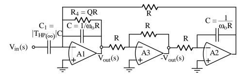
Figure 1-19 - The Tow-Thomas second-order, high-pass active filter realization. Example 1-11 - Design of A High-Pass Filter using the Tow-Thomas of Fig. 1-19
