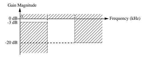
Figure 1-1 - Specification for a low-pass magnitude response in the frequency domain.
