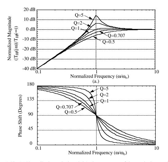
Figure 1-17 - (a.) Normalized magnitude and (b.) phase response of the standard, secondorder, high-pass transfer function with Q as a parameter.
