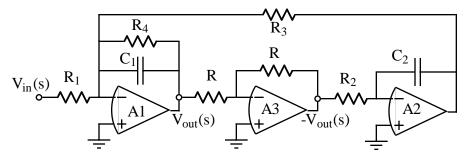
Figure 1-22 - The Tow-Thomas, second-order, bandpass active filter realization. We can show that the transfer function of Fig. 1-22 is given by
