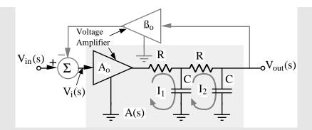
Figure 1-10 - Feedback circuit for Ex. 1-4.
