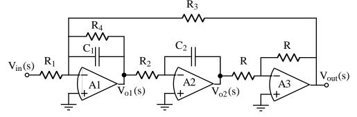
Figure 1-16 - The Tow-Thomas, second-order, low-pass active filter realization.
