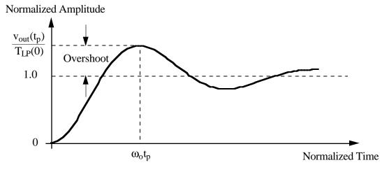
Figure 1-8 - Normalized step response for Q = 2.
