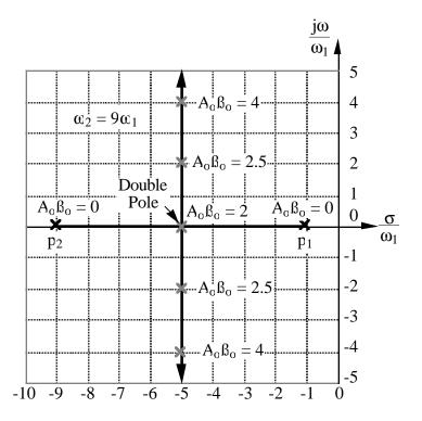
Figure 1-9 - Normalized root-locus of the poles of Eq. (1-19) when  $A_0\beta_0$  is varied from 0 to  $\infty$  for the case where  $\omega_2 = 9\omega_1$ .
