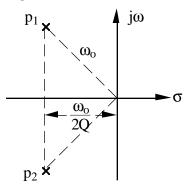
Figure 1-3 - Location of the poles of a second-order system in the complex frequency plane.
