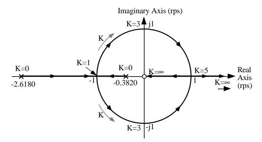
Figure 1-13 - Root locus of the poles of Fig. 1-12a as a function of K.
