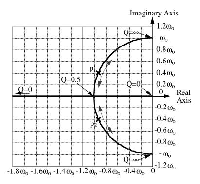
Figure 1-4 - Root-locus of the poles of Eq. (1-3) as Q is varied from 0 to  $\infty$ .
