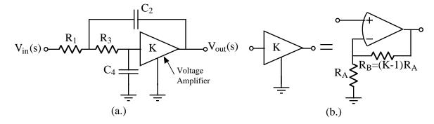
Figure 1-12 - (a.) A second-order, low-pass active filter using positive feedback. (b.) The realization of the voltage amplifier K by the noninverting op amp configuration.
