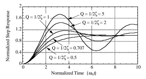
Figure 1-7 - Normalize step response of a standard, low-pass, second-order transfer function for  $Q \ge 5$  (underdamped).
