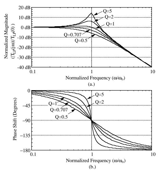
Figure 1-6 - (a.) Normalized magnitude and (b.) phase response of the standard secondorder, low-pass transfer function with Q as a parameter.
