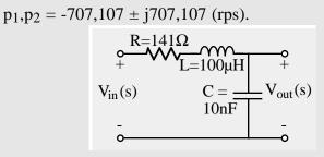
Figure 1-5 - A second-order low-pass RLC filter.
