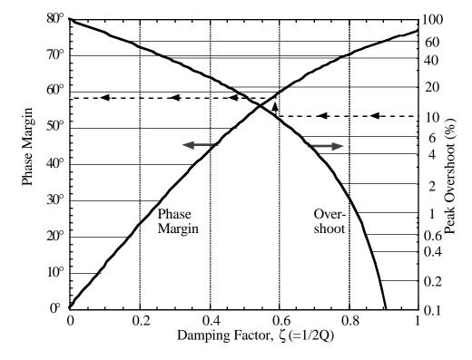
Figure 1-11 - Graphical illustration of the relationship between peak overshoot and phase margin of a negative feedback system.
