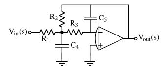
Figure 1-14 - A negative feedback realization of a second-order, low-pass active filter.
