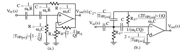
Figure 1-18 - (a.) Positive feedback and (b.) negative feedback, second-order, high-pass active filter realization.
