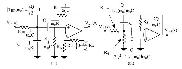
Figure 1-21 - (a.) Positive feedback and (b.) negative feedback, second-order, bandpass active filter realizations.
