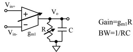
Fig. 1. First-order low-pass  $G_m$ -C filter block diagram.
