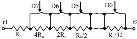
Fig. 10. Tunable, bandwidth-setting resistor R.
